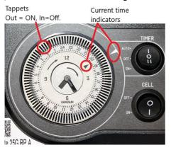
will set the "ON" time, while tappets pushed toward the centre of the clock will set the "OFF" time. Set the current time by turning the outer ring of the clock clockwise until the current time is adjacent to the black and white triangles in line with the "Auto" label. Each tappet represents 15 minutes.
