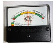
The Chlorine Monitor is an Amp meter and indicates the Chlorine output of your Aquajoy Chlorinator. It does NOT relate to pH control or residual Chlorine in your pool.
