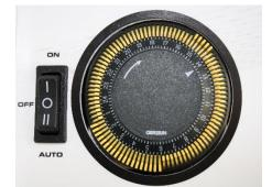
This 24-hour timer controls the Pump / Filter / Chlorinator which is switched ON and OFF by the position of the black tappets. The chlorinator / pump is ON when the black triangle points to the tappets that have been pushed to the outer perimeter of the time face and OFF when the black triangle points to the tappets that are closer to the numbers on the timer face. Each tappet represents 15 minutes.
