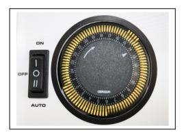
This 24-hour timer controls the Pump / Filter and Chlorinator which is switched ON and OFF by the position of the coloured (White Yellow tappets or depending on age of unit). The chlorinator / pump is ON when the white triangle points to the tappets that have been pushed to the outer perimeter of the time face and OFF when the white triangle points to the tappets that are closer to the numbers on the timer face. Each tappet represents 15 minutes.
