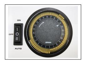
This 24-hour timer controls the Pump / Filter and Chlorinator which is switched ON and OFF by the position of the coloured (White Yellow tappets or depending on age of unit). The chlorinator / pump is ON when the white triangle points to the tappets that have been pushed to the outer perimeter of the time face and OFF when the white triangle points to the tappets that are closer to the numbers on the timer face. Each tappet represents 15 minutes.
