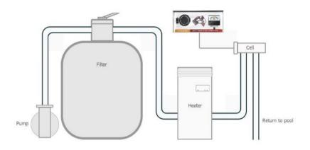
NOTE: WATER MAY FLOW EITHER WAY THROUGH INLET/OUTLET PORTS
